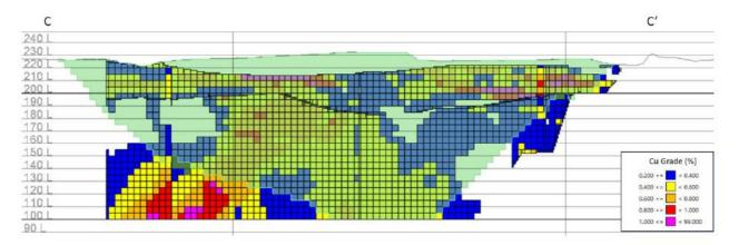
Figure 3. Plan of conceptual Pit 7 and cross-sections and long section showing the final pit outline prior to mine planning and mineralisation based on the MRE reported 9 February 2023 (Source MEC Mining).
