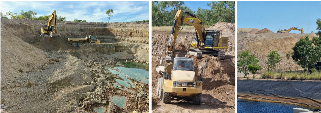
Figure 1. Mining the pit fill and stacking on the heap leach pad.
