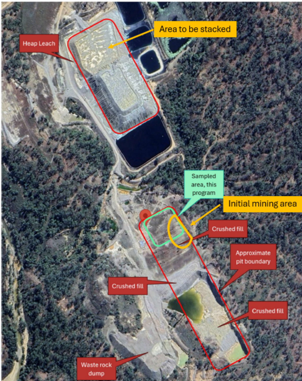
Figure 2. Sampled area in green and the location where initial mining will commence (yellow) to focus on the higher sampled grades. The pit fill is unconsolidated and doesn't require crushing. It was stacked on the lower heap leach pad also outlined in yellow.
