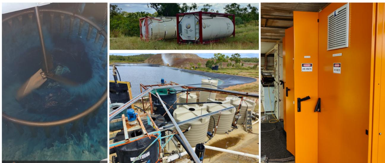
Figure 1. Clockwise. Crystalliser with rotating copper sulphate crystals in suspension, acid tanks awaiting positioning in new bund, new control panel, new tanks and pipework with evaporator in the background.
