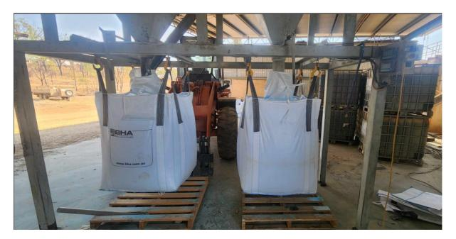
Figure 3. Loading of screened copper sulphate pentahydrate into bulka bags.
