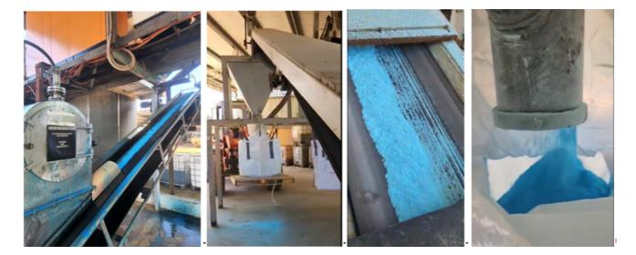
Figure 2. Centrifuge loading conveyer to dryer and bagging
