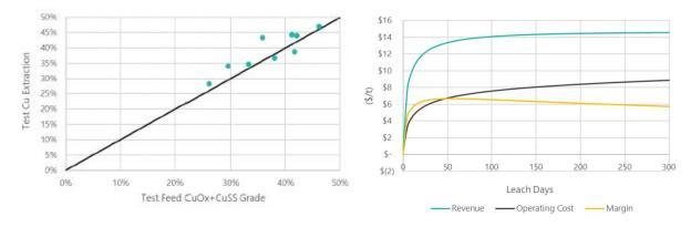
Figure 1(a): Oxide plus secondary sulphide feed grade versus copper extraction. 1(b) Upper leach pad ore revenue, operating cost and margin based on A\$12,700 copper sulphate payable price. Source: TRL002 – Tartana Existing Leachable Copper Estimation of economically-available copper in existing heap and pit fill by Element Process
